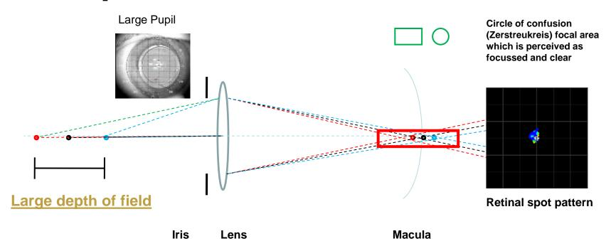
With a large aperture (Iris) a sharp image depends on the optimized curvature (asphericity) of the lens.
